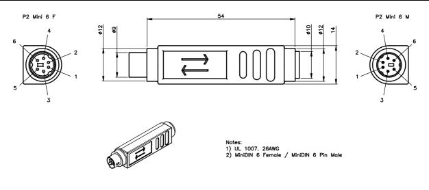
**Note:** Male Connector Pins 1 and 4 are open connections. Female Connector Pins 5 and 6 are open.
